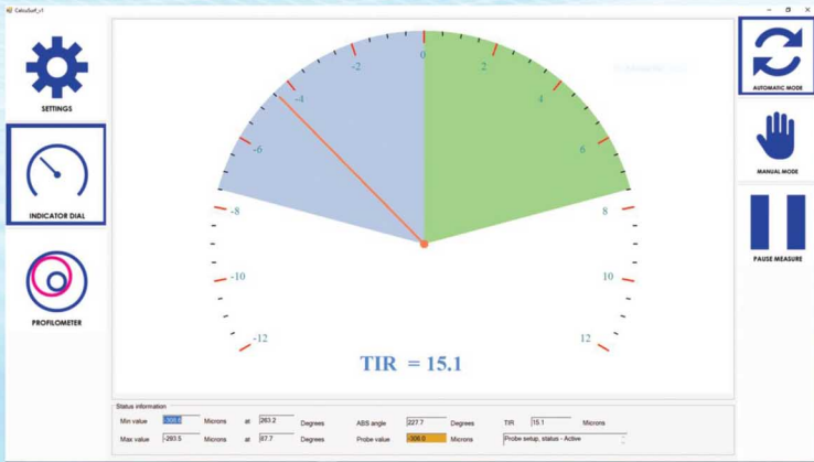
CalcuSurf 2D™ TIR Dial: With realtime auto-scaling function
