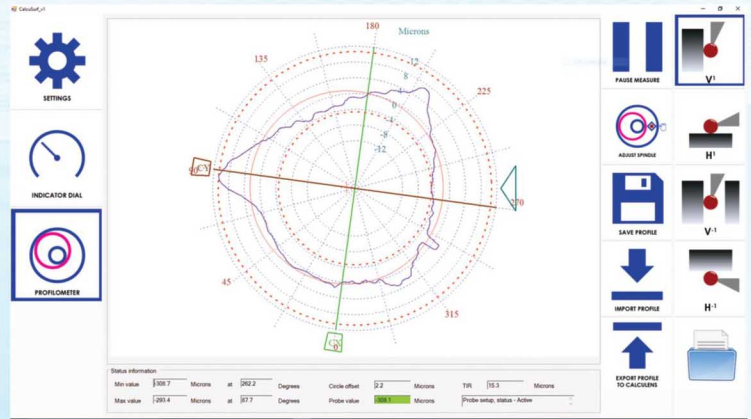
CalcuSurf 2D™ TIR Profile: Best fit circle offset (red cross) Realtime data (purple) Best fit circle (red)
